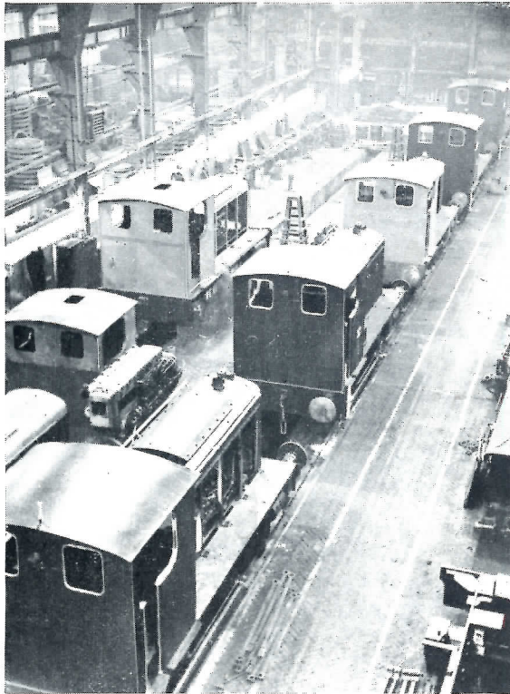
Series of 153 H.P. Locomotives for M.O.S. under erection.
