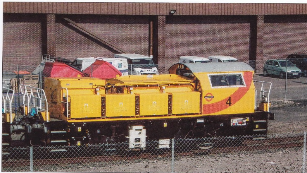
A Schöma London Underground four-wheel diesel hydraulic, after rebuilding in 2015 by Clayton as a battery/ third rail electric locomotive, stands outside the workshop on 24th April 2015. No.4 was Schöma 5406 to become Clayton B4607.04.
