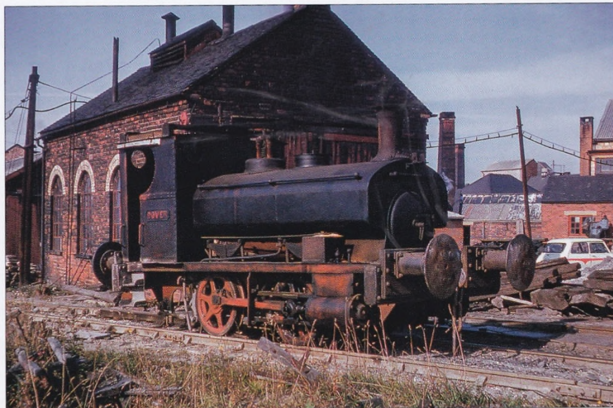
Moving away from Burton, at Leicester Junction, we take the Woodville loop line at Swadlincote Junction on which there were four companies owning locomotives. The one shown here belonged to John Knowles, the pipe manufacturers at Woodville and is Andrew Barclay 891 of 1901 which came to Knowles in 1950 as spare engine after a period at Kings Norton Ordnance Depot.
