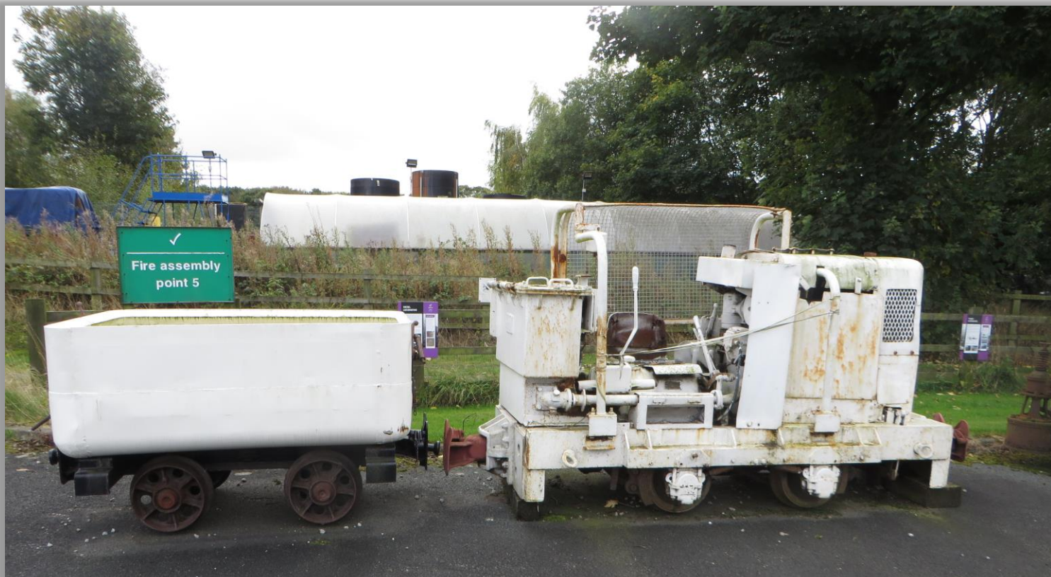
Between 1937 and 1963 Rustons built nearly one thousand, four hundred examples of what might loosely be described as the '20DL family'. Flameproofed 20DLG RH 480679, currently displayed with a mine tub off-track at Caphouse Colliery, was one of the last batch of four delivered between 1961 and 1963.
