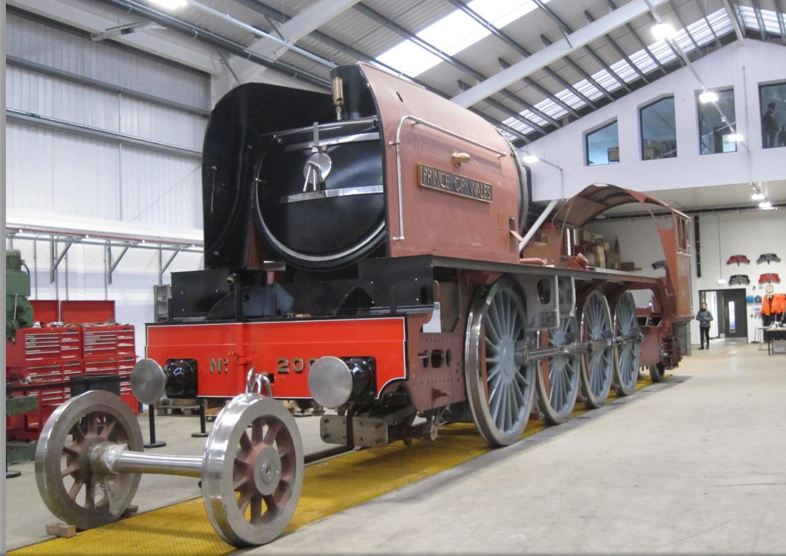
Work progresses on the construction of the P2, although it seems likely to be some time before it is united with its boiler, which currently remains at Meiningen Works, Germany (below, 8 th September).
