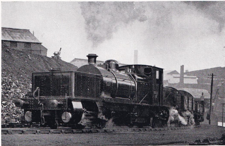
“Garratt” Locomotive and train on 1 in 20 gradient at the Hafod Copper Mills, Swansea.
